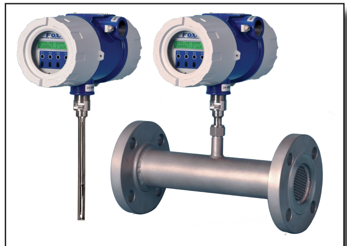
Fox Model FT3 thermal mass flow meter and temperature transmitter. Flow Accuracy: \pm 1\% of reading, \pm 0.2\% of full scale Turndown ratio: up to 1000:1 Available in both insertion and inline styles.
